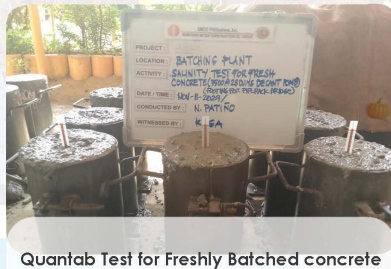
Quantab Test for Freshly Batched concrete
