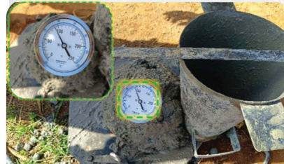
Temperature Test at Site temp: 31° C
