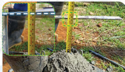
During Slump Test at Site 3500 PSI @ 28 Days Slump: 5 Inch
