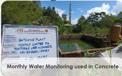
During testing of water using pH paper (pH level of water = 7.6) Tolerance: 4.5 - 8.5 pH
