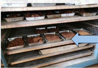
Determine and record the weight of the 6" mold with the compacted sample. Get representative sample from the compacted soil inside the mold for the moisture content. Oven dry the MC samples for each determination
